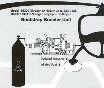
or Helium bottles on helicopters equipped with emergency inflatable "Pop Type" floats \*. However, using either model to service other components needing high pressure Nitrogen such as shock struts and precharging hydraulic accumulators is also common.
